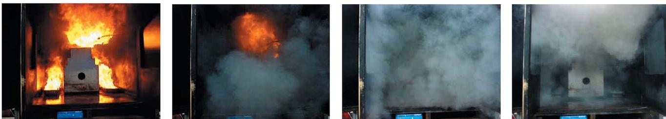
*Pictures are taken at approx. 4-second intervals. The temperature drops during this time from slightly more than +300° C till +40° C. During these 15 seconds, approx 7.5 dl extinguishing fluid is used.*
