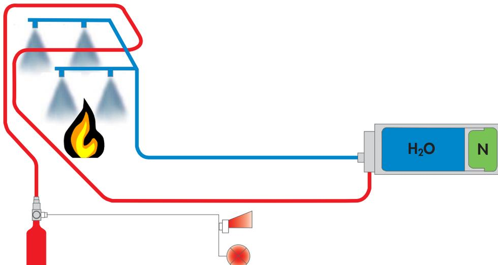
Due to the high pressure of the fogmaker, thick sprinkler pipes are not required, making installation easier.
